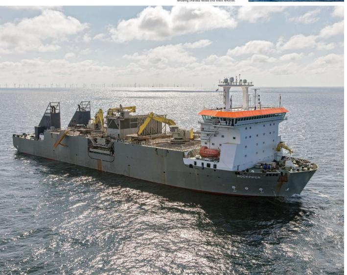
DUTCH SECTOR, NORTH SEA Fallpipe vessel Rockpiper installing rocks that will protect the 67 kilometer long export cables connecting the Borssele offshore wind farm to the Dutch onshore power grid.
